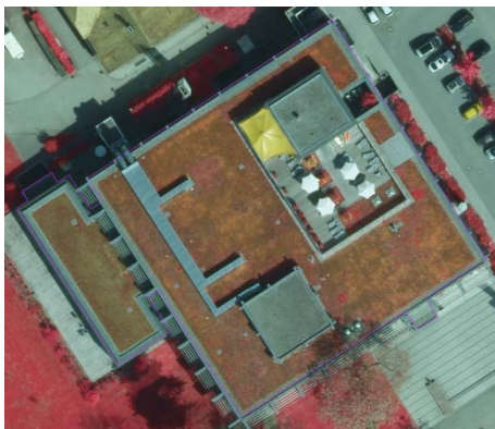
Fig. 1: The green roof detection tool combines high resolution airborne infrared imagery (false color, vegetation in red) and building outlines (purple frame). © City of Nuertingen
